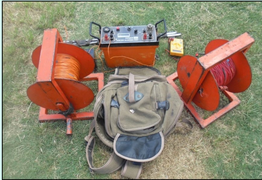
Figure 6: ABEM Terrameter instrument for Geophysical Electrical Resistivity Survey.
